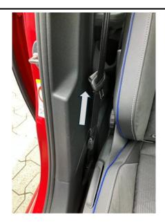
Please firmly pull on the belt webbing of the lower anchoring point in the direction of the arrow (see illustration) on the front passenger seat.
