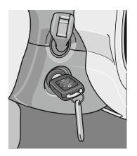
Turn the ignition key to the "OFF" position and remove it.
