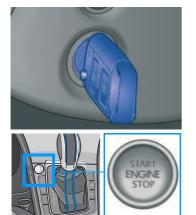
1. Turn the ignition key to the "OFF" position and remove it or press the START/STOP button.
